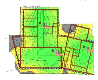
wood? Which insulation material has been used? Which buildings are in your immediate vicinity? Is your company located in the city or in the countryside? On the basis of the collected parameters, we determine how many access points are required for a full coverage.
